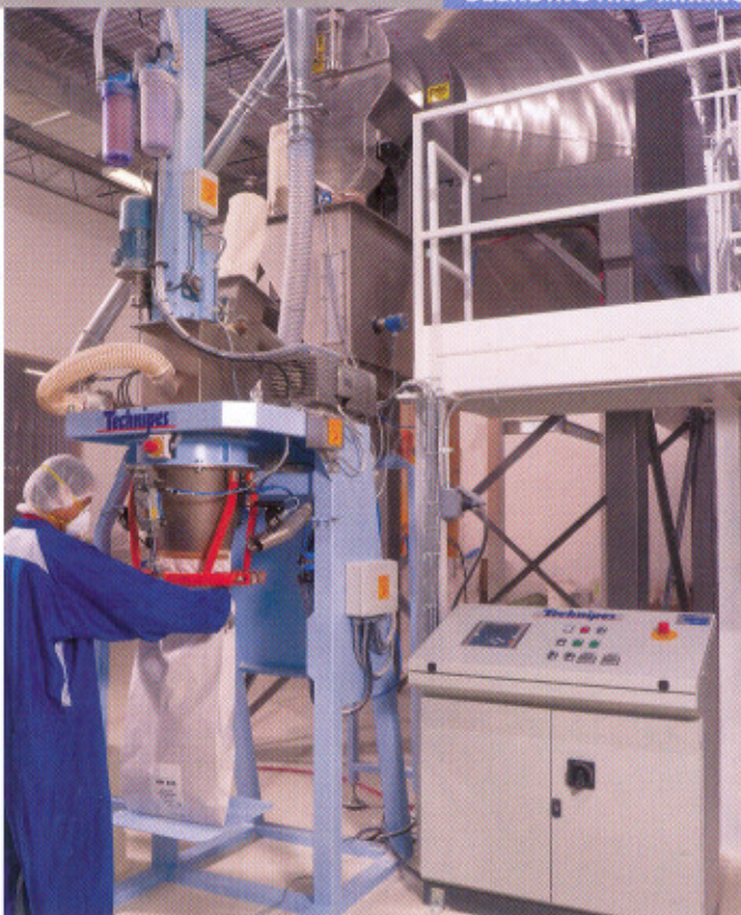
Powders discharge from mixer into hopper and then to bagging machine, which fills 25 kg bags or 1,000 kg bulk bags.
