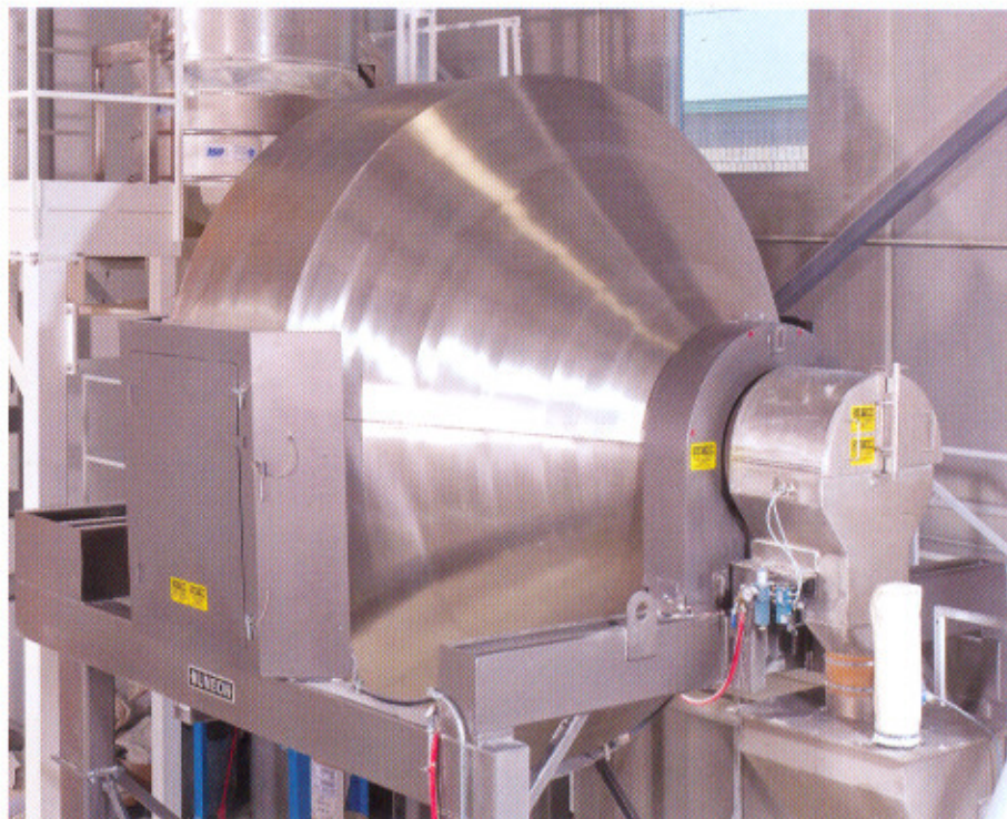
Upon discharge, the 3.96 cu m capacity rotary batch mixer evacuates completely, says Munson, with little or no residual, allowing fast, thorough cleaning between batches. Continuous rotation of the drum assures that all materials remain in motion, preventing segregation in batches of varying material densities.
